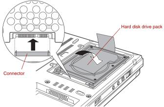
Figure 3-21 Installing the hard disk drive pack
